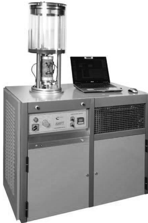
Fig. 1 Equipment to measure the complex modulus of asphalt concrete using the TP 62 and AMPT standard test methods
